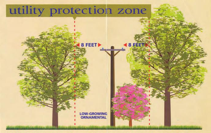
Our vegetation management plan seeks to create a ground-to-sky "Utility Protection Zone" extending 8 feet horizontally from the outermost electrical conductor or wire installed from pole to pole.
